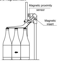
In case of problem (example bottle downing) the control contact lever lowers and magnetic sensor detects the presence of magnetic insert and stops the conveyor.
