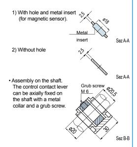
Assembly of Part. S0518 (with insert for magnetic sensor)
