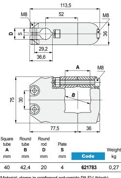
Material: clamp in reinforced polyamide PA FV (black), tightening screws in austenitic stainless steel, nuts in nickel plated brass.
