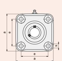
• Series UCF • Type B Grub screws shaft locking
